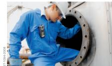
Dräger X-am® 2500 Reliable personal protection, e.g. in confined space entry.
